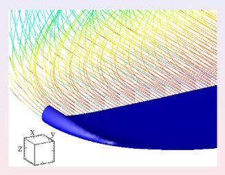
Figure: The local 3D vortex structures and vortex lines around the maximum vorticity at t=17.
