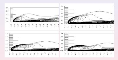
Figure: The contour of axial vorticity around the maximum vorticity on the symmetry plane (the xz-plane) at t=17.5,18,18.5,19.
