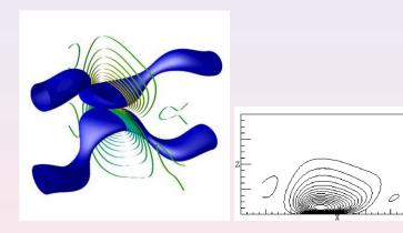
Figure: The 3D vortex tube and axial vorticity on the symmetry plane when t=6.
