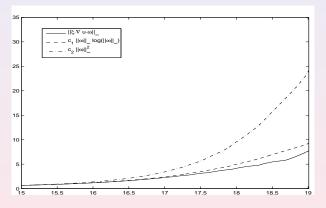
Figure: Study of the vortex stretching term in time, resolution  $1536 \times 1024 \times 3072$ . The fact  $|\boldsymbol{\xi} \cdot \nabla \mathbf{u} \cdot \boldsymbol{\omega}| \leq c_1 |\boldsymbol{\omega}| log |\boldsymbol{\omega}|$  plus  $\frac{D}{Dt} |\boldsymbol{\omega}| = \boldsymbol{\xi} \cdot \nabla \mathbf{u} \cdot \boldsymbol{\omega}$  implies  $|\boldsymbol{\omega}|$  bounded by doubly exponential.
