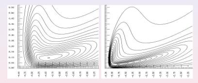
Figure: The contour of axial vorticity around the maximum vorticity on the symmetry plane at t=15,17.
