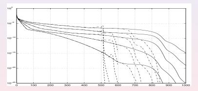
Figure: The enstrophy spectra versus wave numbers. The dashed lines and dashed-dotted lines are solutions with  $768 \times 512 \times 1024$  using the 2/3 dealiasing rule and the Fourier smoothing, respectively. The times for the spectra lines are at t=15,16,17,18,19 respectively.
